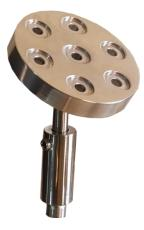
The device can be equipped with different sample stage configurations depending on the user requirements. The sample stages are rotatable with adjustable height and easy to change.
