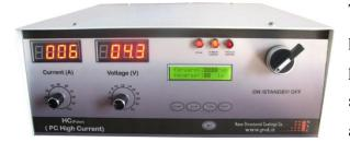
The Desk vacuum carbon coater is able to perform pulsed carbon fiber evaporation. Short pulses provide more controlled deposition and significantly reduces the amount of debris associated with traditional carbon deposition.
