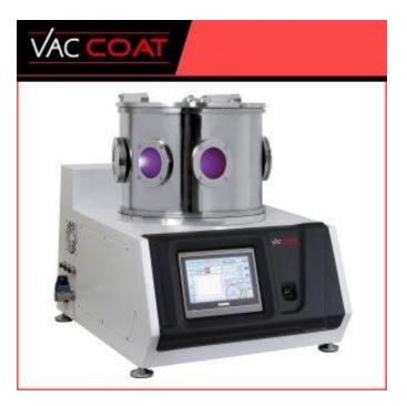
PLD – T is a high vacuum thin film deposition system enables to deposit different materials by both Pulsed Laser Deposition and thermal evaporation technique. It can deposit complex materials and crystalline structures onto substrates with very little setup involved.
