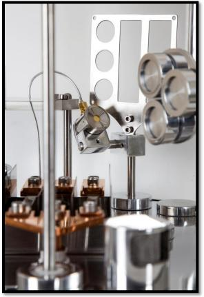
PLD – T is equipped with a multi-target manipulator which includes three 2 cm diameter. Targets are in standard size.
